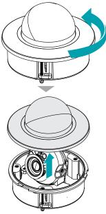
Turn the camera body counterclockwise while 2 pressing the body hook of the bottom cover to remove from the bottom cover.
