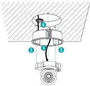
7 Connect the camera body to the bottom cover. Match the cable access hole position of bottom cover and camera body as the following image and turn the camera body clockwise to fix it.
